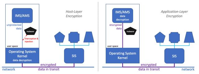
Figure 9. While host-to-host encryption (left) protects against network-based attacks, it does not protect against co-resident malware on an IMS/AMS. Malware can be installed on the platform through trojan DTM installers and other social engineering and lifecycle attacks. Application layer encryption (right) is necessary to protect against malware with this vantage point.
