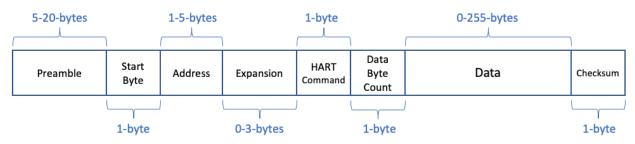
Figure 6. The request HART packet structure has a preamble field (for synchronization and carrier detect), a start delimiter (that designates the start of the communications packet), the device address, an expansion field, a numerical value designating a HART command, a size field for the data, a data field, and a 1-byte checksum for packet integrity.
