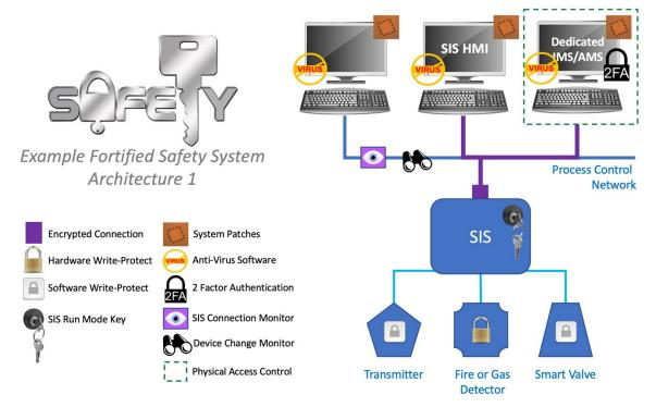
Figure 8. Manage risk by implementing a layered, defense-in-depth approach that fortifies safety systems and their operating environments against network-based, insider, and supply-chain attacks.
