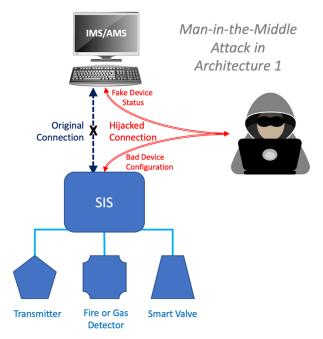
Figure 7. Under certain conditions, unencrypted communications can be hijacked by attackers and used to block or change operator-initiated device commands and send false device status to the IMS/AMS operator console. Using alternate techniques, a similar capability could be achieved through co-resident malware running directly on the IMS/AMS.
